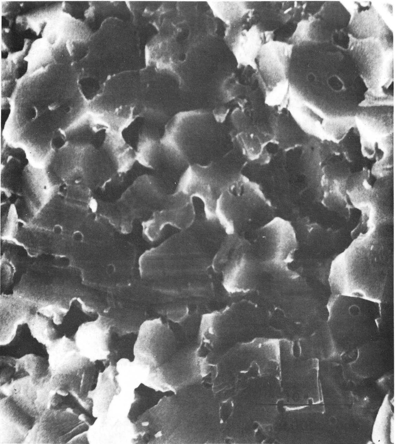
Fig. 26. Fracture surface of MgO sintered at 1510°C for 700 min in flowing water vapor.
