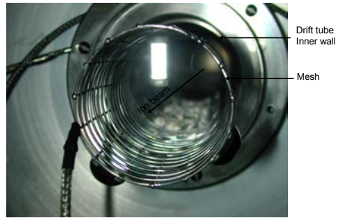
FIG.5. Cylindrical metal mesh of outer diameter 6.3 cm was installed inside a 7.6 cm diameter beam drift tube.
