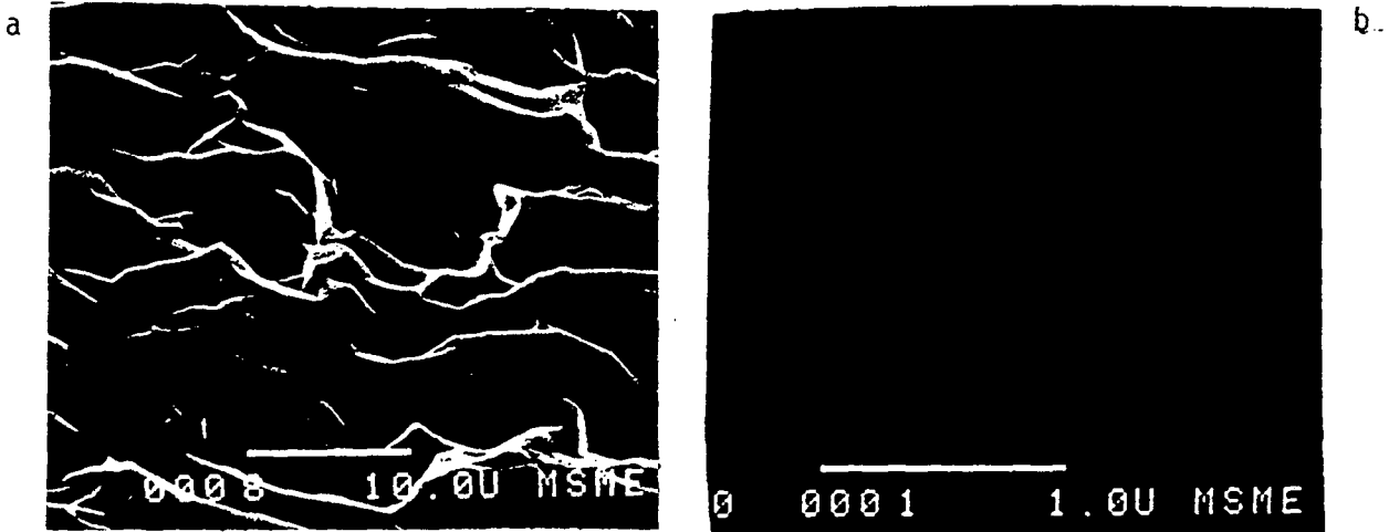
Figure 3 SEM micrographs of an \text{Al}_2\text{O}_3 thin film ( 2000\text{\AA} ) deposited on silicon. (a) without magnetic filter. (b) with magnetic filter for the formation of high purity and smooth thin films
