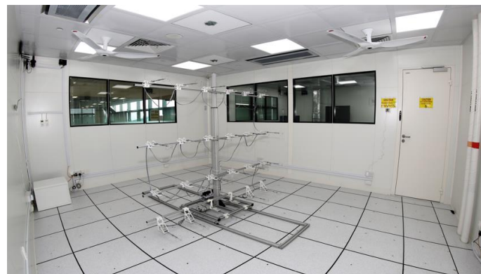
Figure 2. Climatic chambers for air speed measurement: anemometer sensor tree.
