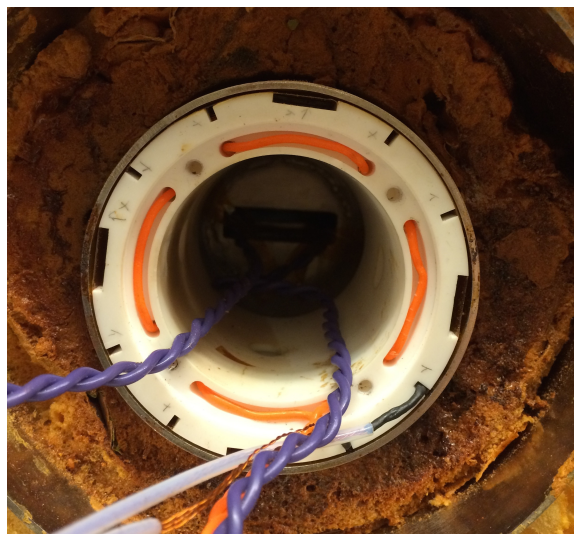
Figure 3.6: Photograph of Phase-II magnetometer inner shields and coil housing.
