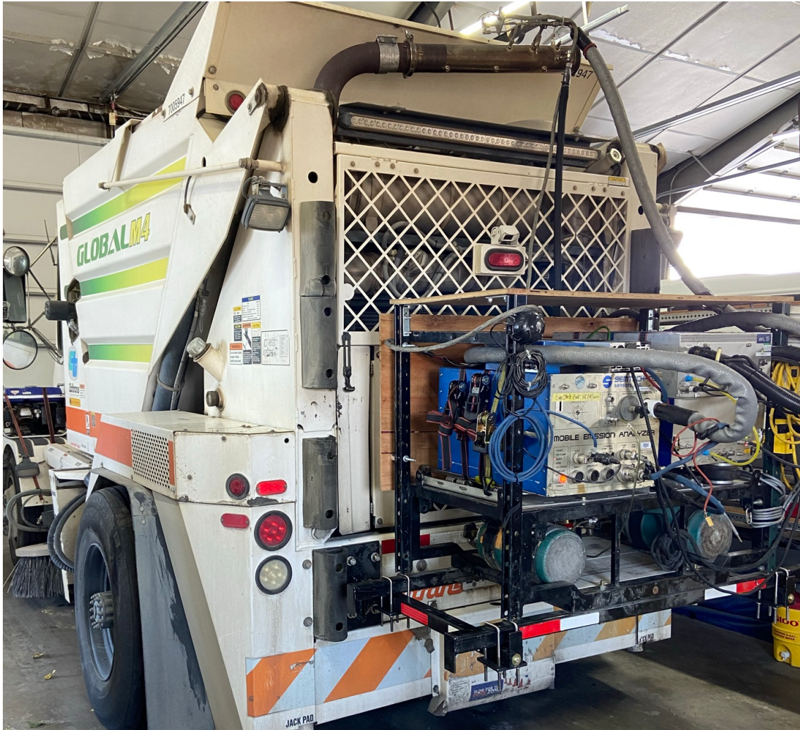
Figure 2-5: PEMS rack installed on street sweeper
