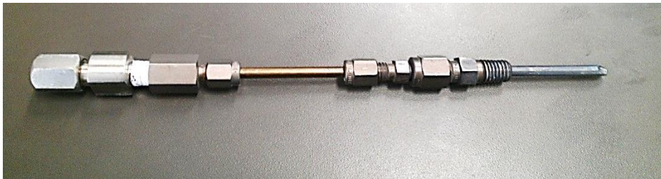
Figure 2-3: Sample holder that is inserted from the back of the autoclave and can hold up to 2 electrodes in one holder
