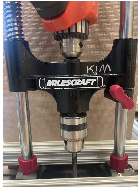
Figure 4.1: Spring loaded drill rig
