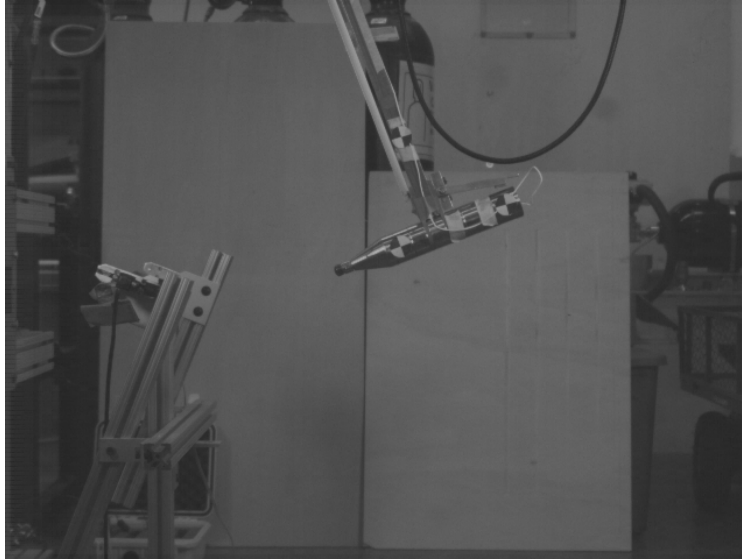
Figure 4.5: In-situ pendulum impactor during PE to KE transition
