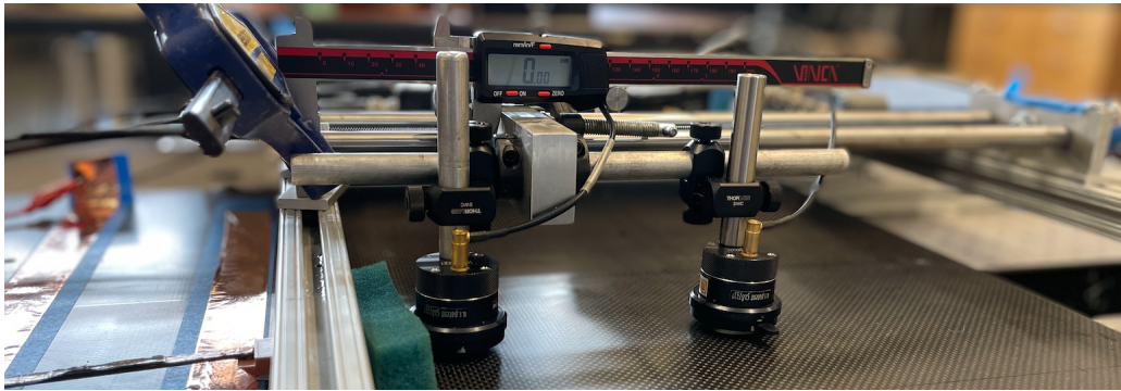
Figure 4.19: Fabricated Linear Stage Translator at the Origin. A digital caliper is used to precisely locate the broadband acoustic transducers along the scan path. Note the 8ply-88mm impactor to the left
