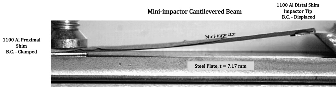
Figure 2.1: A representative mini-impactor. The mini-impactor is clamped to a steel plate and mini-impactor's tip is displaced normal to the plate to a height of 6.35mm.
