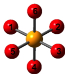
Figure 6. First coordination sphere around Fe for all the species except A. Atoms O1–O5 are the five MOF oxygen atoms around the Fe center, and O6 is the oxygen atom transferred from N 2 O to the iron center. [Color code: Orange = Fe and red = O].
