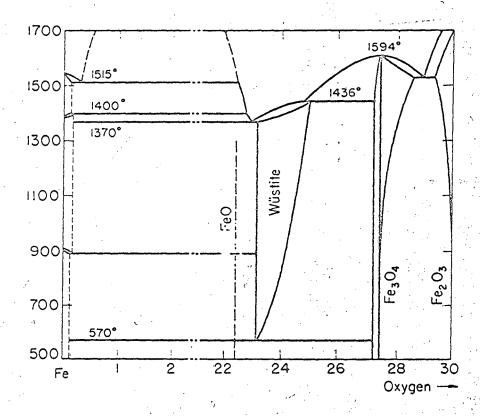
Fig. 1. The Fe-Fe<sub>2</sub>0<sub>3</sub> phase diagram.
