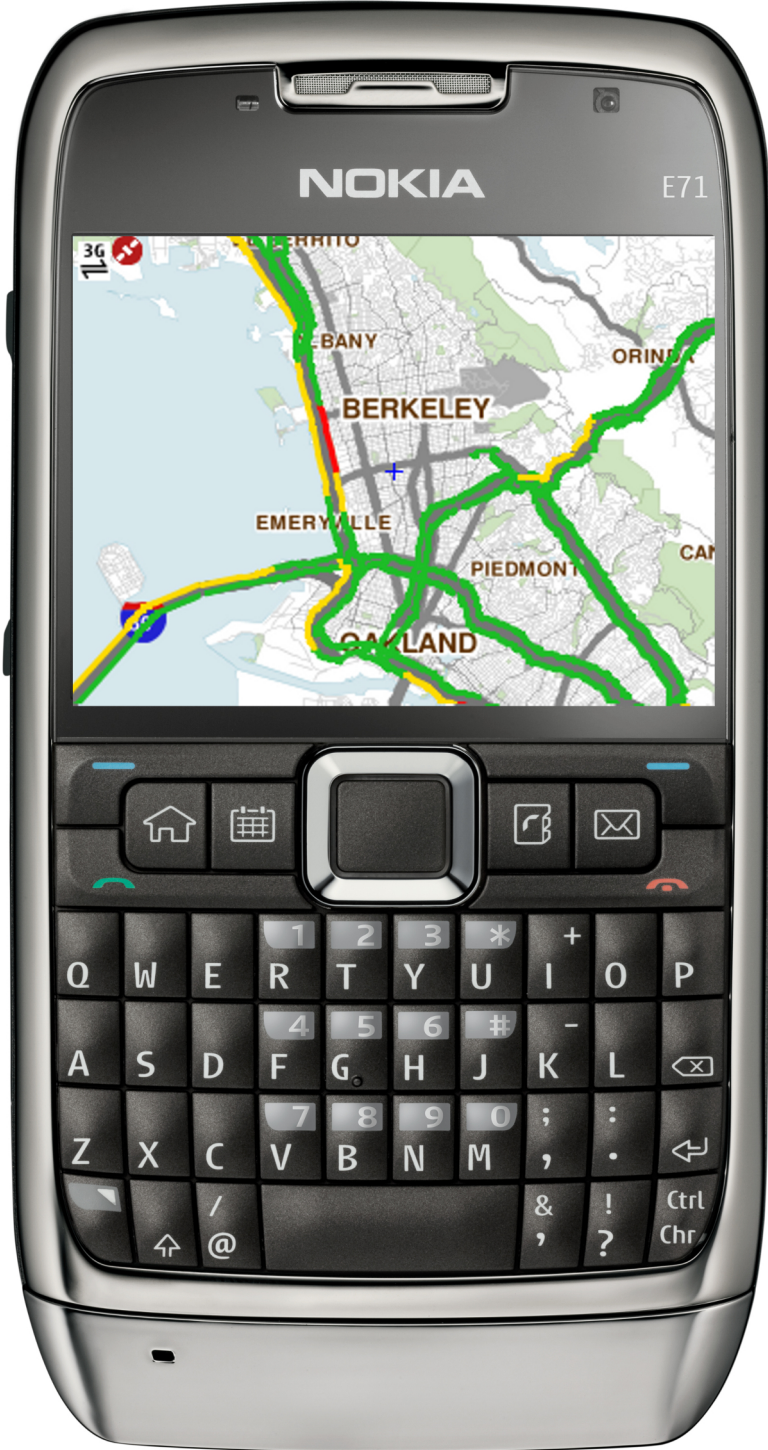
Figure 2.9: The Mobile Millennium phone client running on a Nokia E71. The phone client displays a color map of current traffic conditions around the driver’s location while simultaneously providing VTL data to a central server.
