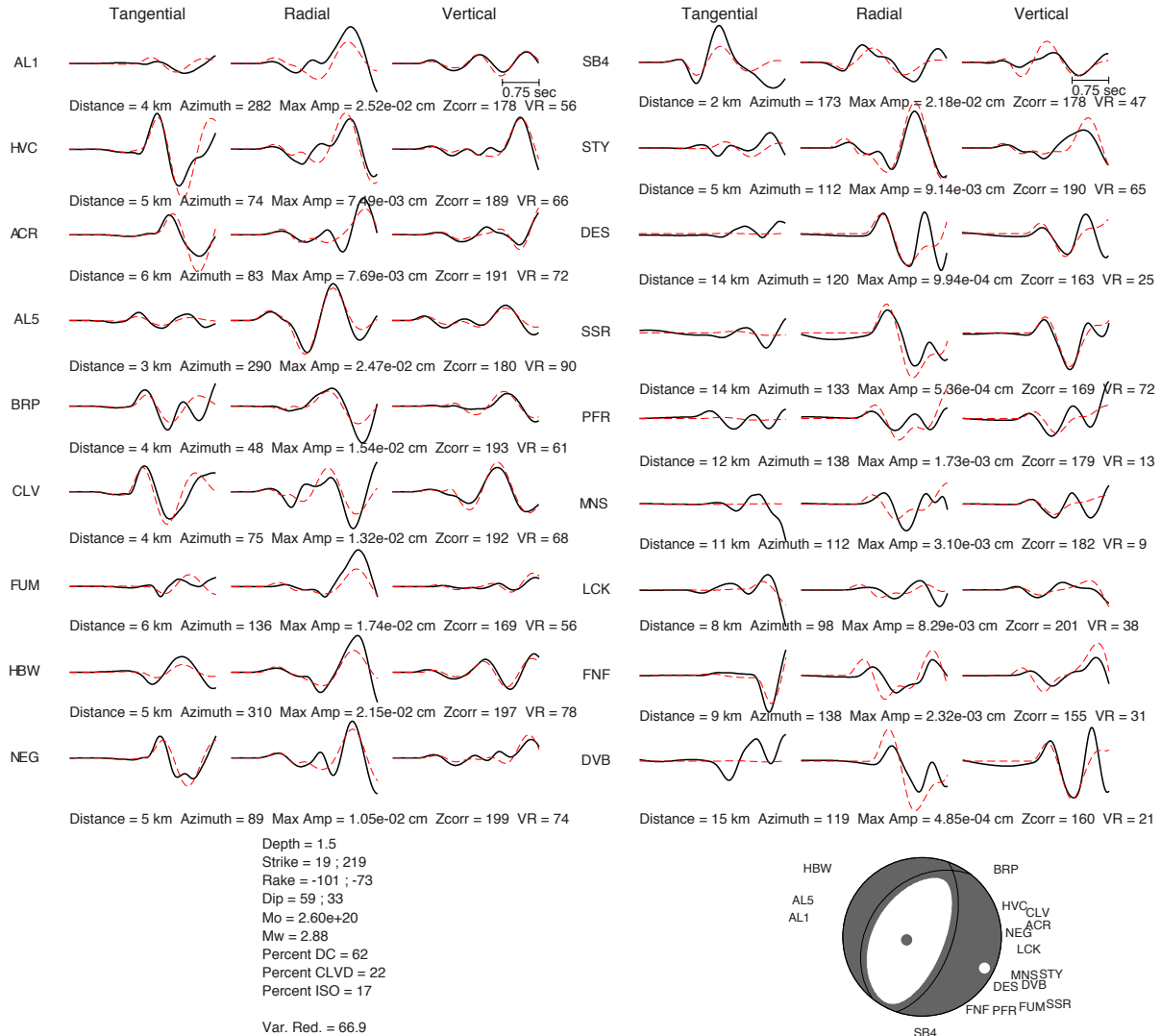
Figure 23. Comparison of filtered (0.2 to 1.0 Hz) observed velocity data (black) and synthetic (red) waveform fits and P -wave radiation pattern of the full moment tensor solution for target event 4, M_W 2.87 February 6, 2013. The improvement in fit of the full moment tensor solution is 0.3% and is too small to be statistically significant. Gray and white dots represent pressure and tension axes, respectively.
