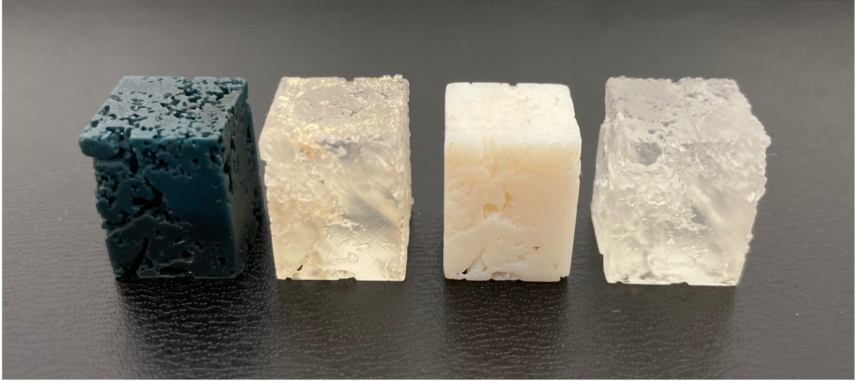
Figure A.6: Photograph of the produced printed soil analogues by DLS, PJ Gel, LFS, and PJ WS, arranged left to right.
