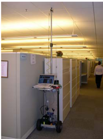
Figure 4a Commissioning cart with extended mast
