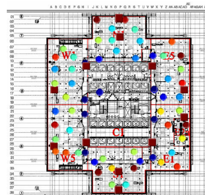
4c Screen shot of supply air temperatures (round) and mid-level room temperatures (squares)
