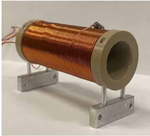
Figure 4: Assembled solenoid mounted on PEEK enclosure.
