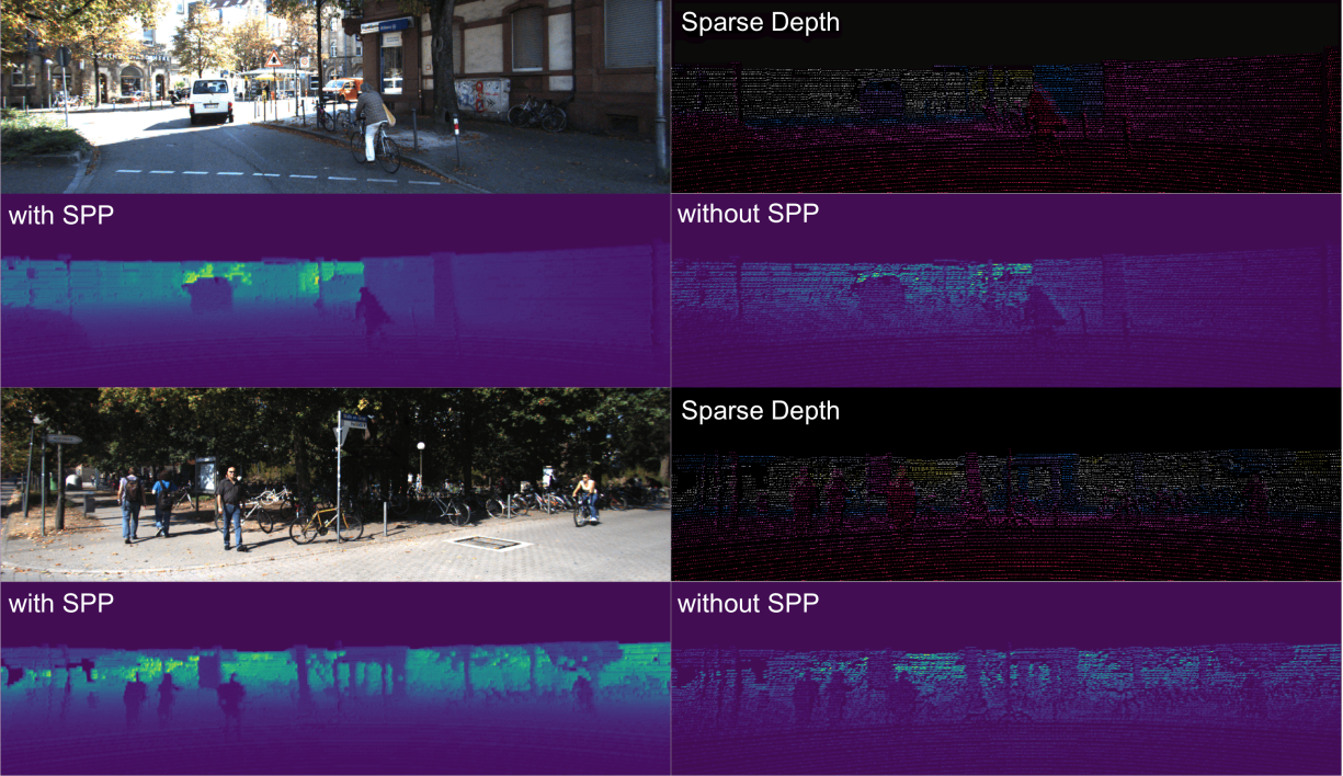
Figure 7.7: A comparison of feature maps produced by ScaffNet with and without Spatial Pyramid Pooling (SPP). Hidden layer outputs (feature maps) after 5 \times 5 convolutional layers with and without SPP. The feature maps produced by ScaffNet without SPP are sparse and resembles the input sparse depth, which illustrates our claim – neurons are not activated because of the missing sparse depth measurements. In contrast, when using SPP, ScaffNet produces a much denser representation.
