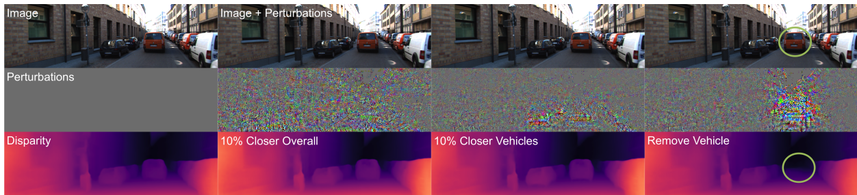
Figure 8.1: Altering the predicted scene with adversarial perturbations. Top to bottom: input image; adversarial perturbations with upper norm of 2 \times 10^{-2} ; predicted scene visualized as disparity. Left to right: original image and predicted scene; overall scene altered to be 10% closer; all vehicles altered to be 10% closer; vehicle in the center of the road is removed by perturbations.
