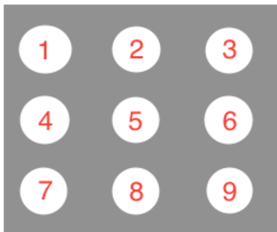
Figure 4.1. Nine indium foils. Foil 5 is at the origin. The z-axis, defined by the direction of the deuteron beam, passes through the center of foil 5 perpendicular to the plane.
