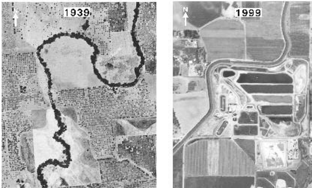
Figure Two: Example of restructuring and channelization of Marsh Creek for flood control. Note lack of channel form diversity and loss of channel length.
