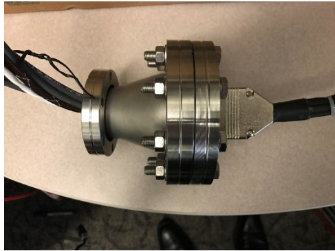
Figure 29: 25-pin D-Sub interface flange for the TVAC chamber.
