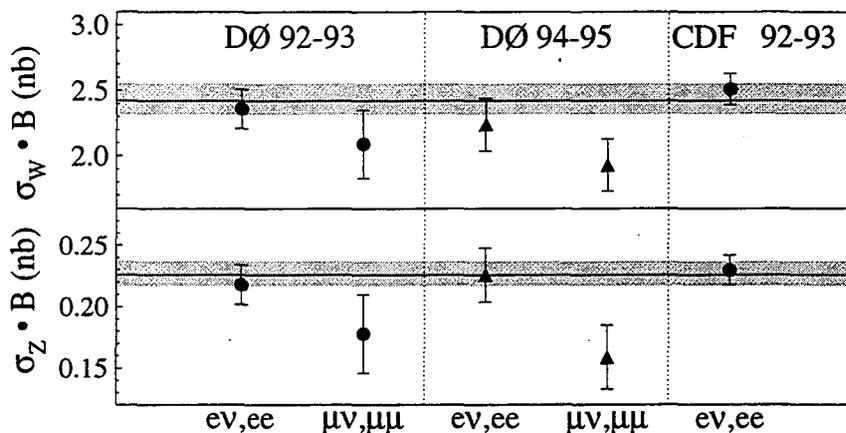
FIG. 4.  $\sigma \cdot B$  for inclusive  $W$  and  $Z$  boson production from DØ and CDF for the 1992–93 data and preliminary results from DØ from part of the 1994–95 data. The error bars indicate the combined statistical and systematic errors. The solid lines are the predicted values calculated using the CTEQ2M pdf and the shaded bands indicate the uncertainty in the predictions.
