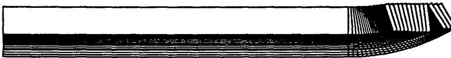
Figure 14 Conductor geometry in the end region of the SSC quad — LAYER-2 SIDE.
