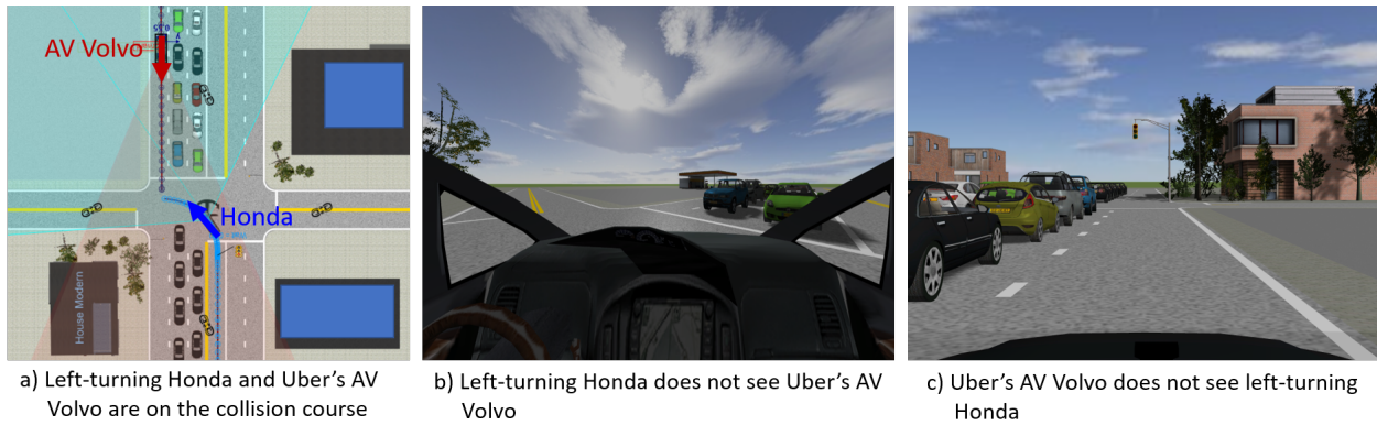
Figure 2.2: PreScan simulation of V_1 and V_2 collision—snapshot of the scenario 2 seconds before the accident.
