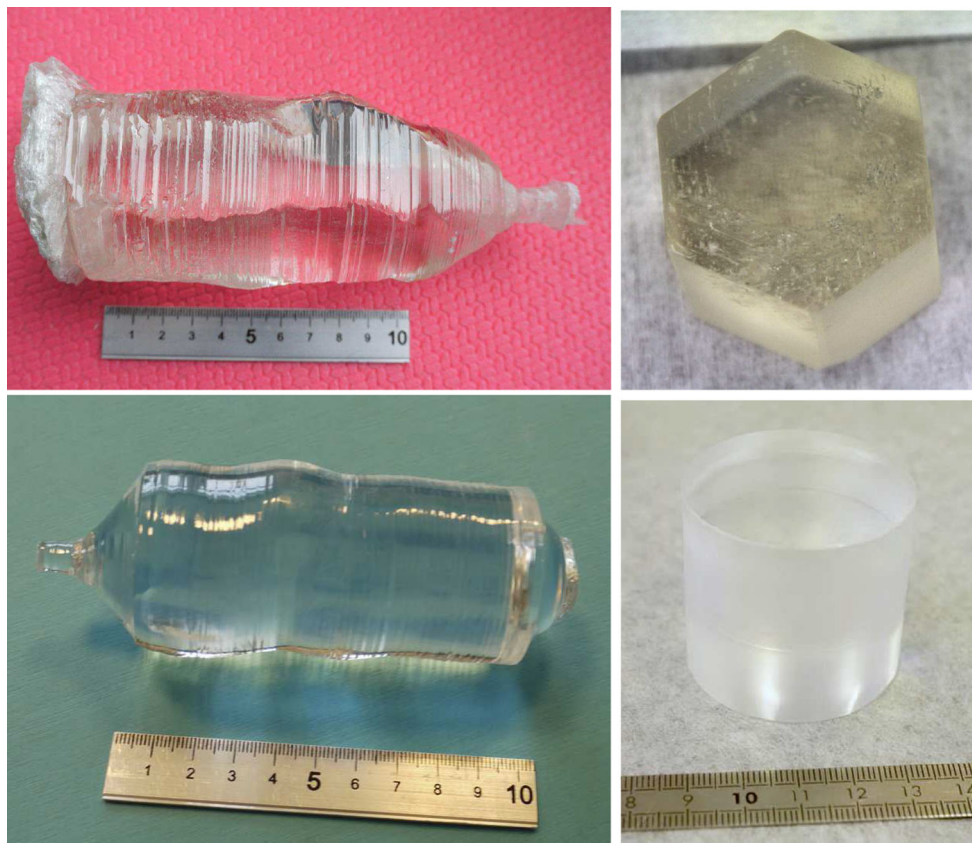
Fig. 1 Photographs of the first large-mass ^{100}\text{Mo} -enriched scintillators: the \sim 1.4 kg \text{Zn}^{100}\text{MoO}_4 crystal boule with the cut \sim 0.38 kg scintillation element enrZMO-t (top panels), and the \sim 0.5 kg boule of \text{Li}_2^{100}\text{MoO}_4 crystal with the produced \sim 0.2 kg sample enrLMO-t (bot-
