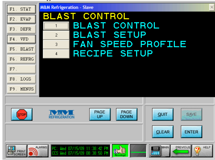
Figure 11: Blast Freezer Control Screen
