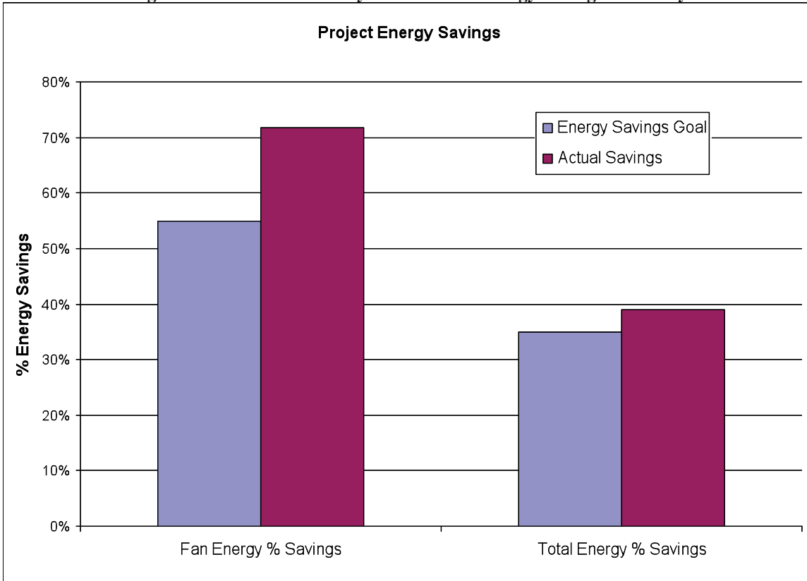
Figure 33: Standard Blast Cycle Run Time Energy Savings Summary
