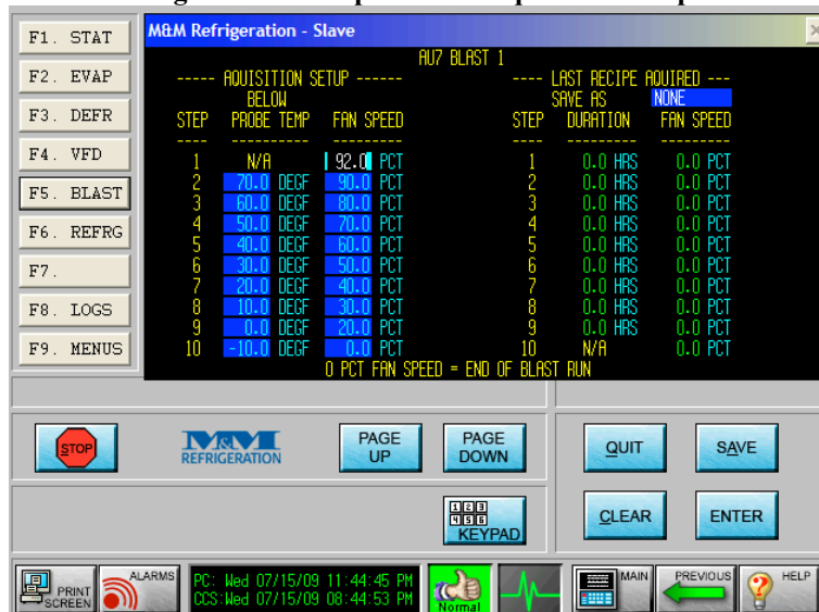
Figure 15: Fan Speed and Acquisition Setup
