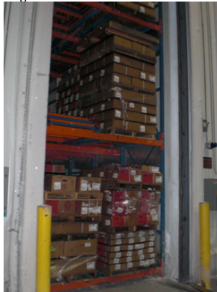
Figure 1: Front View of a Blast Cell
