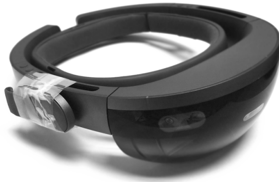
Figure 2.2: HoloLens 1 with a clicker tapped to the side. Pressing the clicker was faster and more accurate than hand gestures.
