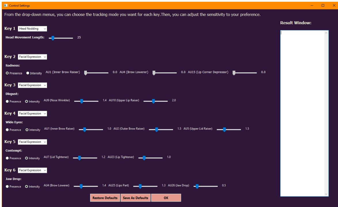
Figure 3.3: We built a custom interface to enable users to change AU detection thresholds and head nod distance.
