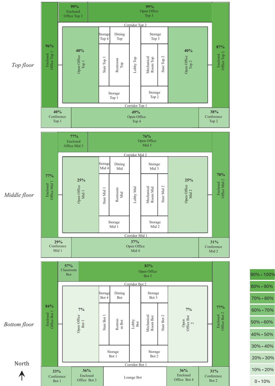
Fig. 5 Color-coded cold thermal discomfort rating in the top, mid, and bottom floor plans for the pre-1980 vintage office building under power-interrupted extreme cold snap event in 2023
