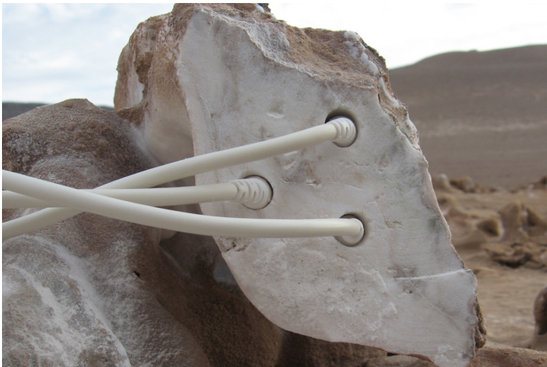
Figure 3. Installation of temperature and relative humidity sensors within the halite nodules at each site. Sensors were installed directly into the side of nodules at the Qh site (a), and installed deeper within the nodule at the Qp site (b) after section the nodule with an electric saw. Approximate size of sensor is 1 cm diameter.
