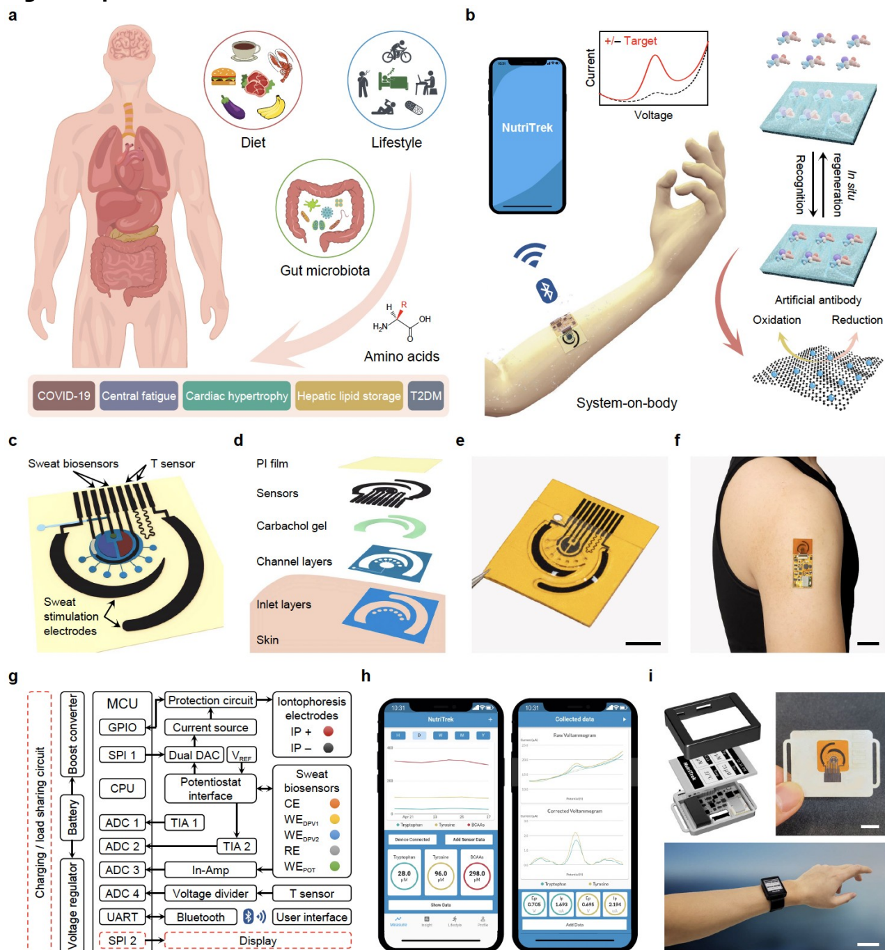
Fig. 1 | Schematics and images of the wearable biosensor 'NutriTrek'. a , Circulating nutrients such as amino acids are associated with various physiological and metabolic conditions. b , Schematic of the wearable 'NutriTrek' that enables metabolic monitoring through a synergistic fusion of laser-engraved graphene, redox-active nanoreporters, and artificial. c,d , Schematic ( c ) and layer assembly ( d ) of the microfluidic 'NutriTrek' patch for sweat induction, sampling, and biosensing. T, temperature; PI, polyimide. e,f , Images of a flexible sensor patch ( e ) and a skin-interfaced wearable system ( f ). Scale bars, 5 mm ( e ) and 2 cm ( f ). g , Block diagram of electronic system of 'NutriTrek'. The modules outlined in red dashes are included in the smartwatch version. ADC, analog-to-digital converter; DAC, digital-to-analog converter; CPU, central processing unit; GPIO, general-purpose input/output; POT, potentiometry; In-Amp, instrumentation amplifier; MCU, microcontroller; SPI, serial peripheral interface; TIA, transimpedance amplifier; UART, universal asynchronous receiver-transmitter; IP, iontophoresis; CE, counter electrode; RE, reference electrode; WE, working electrode; DPV,
