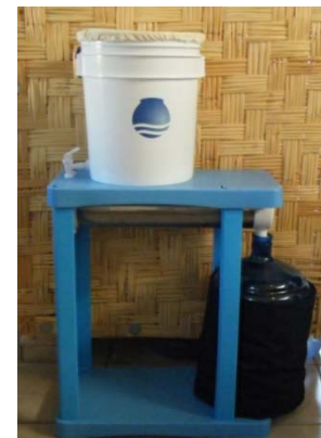
The height is set to fit the garrafon and separate it from the ground.
