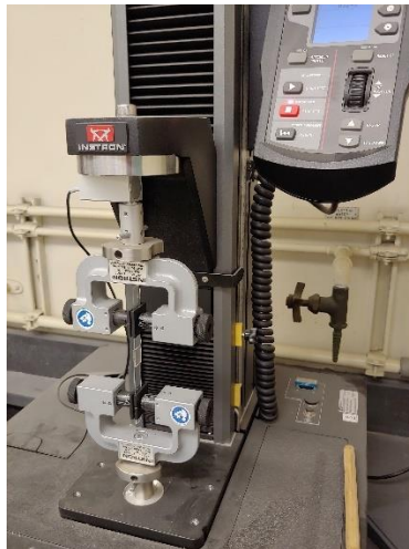
Figure 2.1: The Instron 5942 with the installed 100 N load cell and a sample mounted in place.
