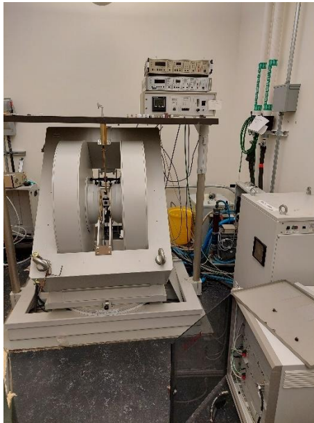
Figure 2.8: The Bruker EMX EPR instrument at UC Riverside used in the experiments. The magnet and resonator cavity are visible in the middle, the temperature control is above the magnet. The power supply for the magnet and transputer are on the front right of the image. The X-band microwave generator is absent from the picture as it was being repaired at the time. The dewar for the cryogen is behind the instrument.
