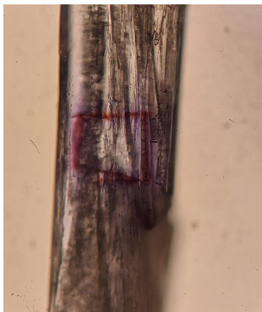
Figure 5.10: Spatial patterning of nitrenes into a single crystal of 4F4ABC leaves a purple square where the sample was exposed to 405 nm light. Similar results are obtained with 365 nm light.
