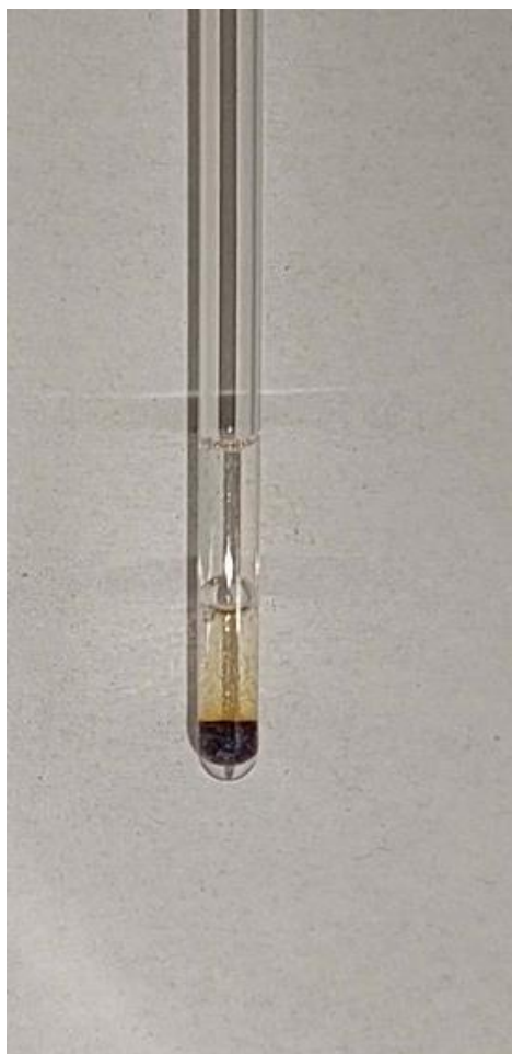
Figure S5.12: A photo of 4F4ABC dissolving in acetone. Small and large bubbles can be seen evolving from the sample. The dissolving portions are turning brown as the nitrene is reacting.
