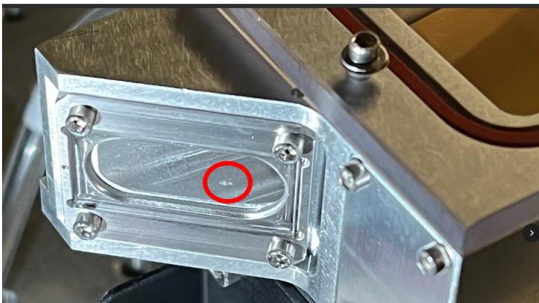
Figure 2.6 Damaged optics in the laser system that must be replaced. (a)The input window of the RGA crystal chamber (b) the compressor grating.
