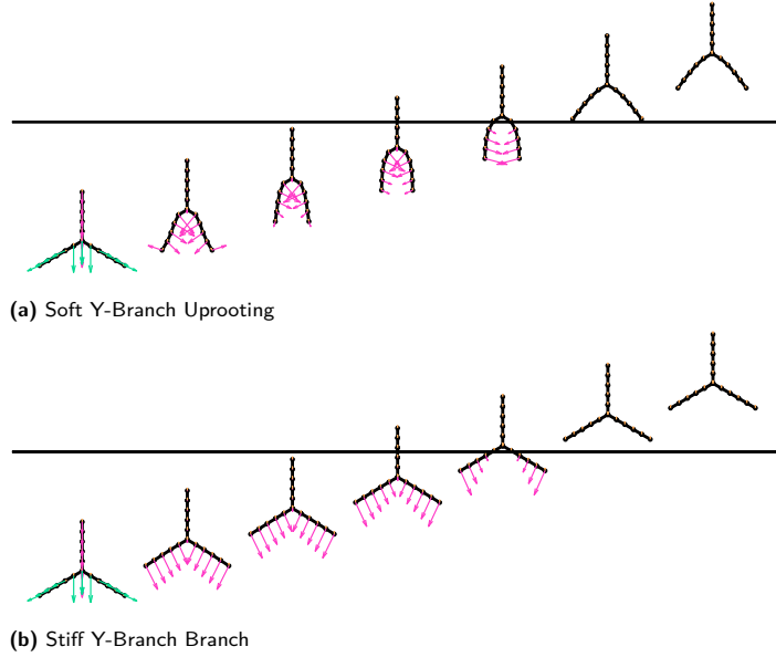
Fig. 13 Response of identical roots with different material properties to constant velocity pull at the top node with gravity.
