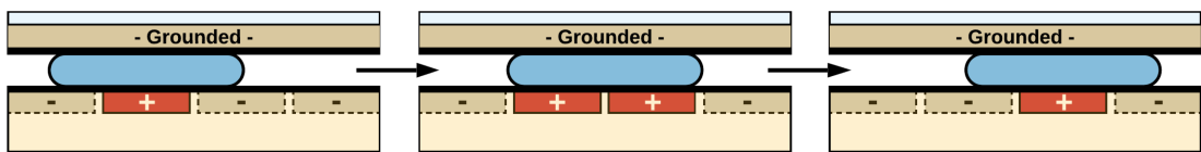
Figure 2.2: Droplet transport is achieved by activating and deactivating electrodes in sequence.
