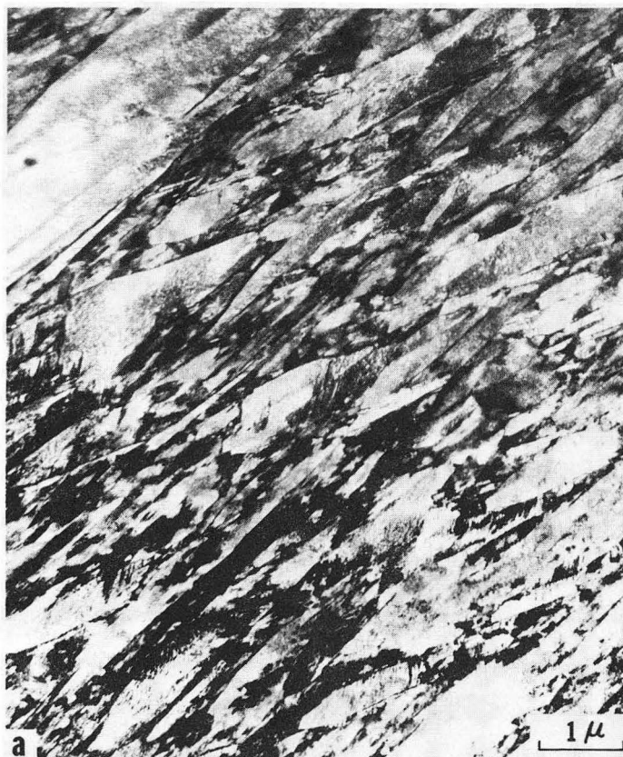
Figure 10 Transmission electron micrographs of as-quenched AISI 4340 steel: (a) bright field and (b) dark field of an austenite spot for the high-austenitizing treatment.
