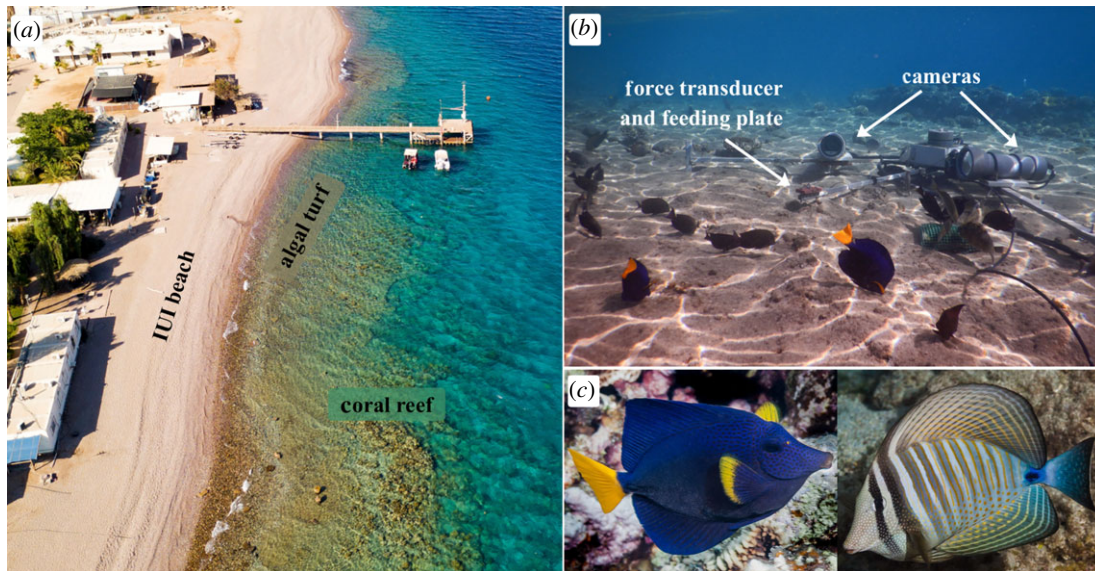
Figure 1. Documenting in situ feeding kinematics of herbivorous reef fishes feeding in the Red Sea. (a) An aerial view of the fringing reef and algal turfs at the study site, the Interuniversity Institute for Marine Sciences (IUI) in Eilat, Israel. (b) The underwater video system, positioned on the algal turf, was comprised of two high speed cameras and a synchronized force transducer. The system allowed the three-dimensional tracking of the movements of the fish's body, fins and mouth during feeding, while simultaneously measuring the forces they exerted on a feeding plate naturally colonized by turf algae. (c) We focused on two species of Acanthuridae, Zebrasoma xanthurum (left) and Zebrasoma desjardini (right), both characterized by a deep body shape, elongated dorsal and anal fins, protruding snout and a small mouth, as well as serrated teeth that allow them to tear algae. Photos by (a) Yoav Lindman and (c) François Libert. (Online version in colour.)
