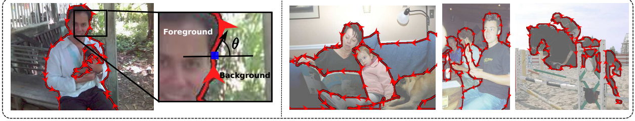
Figure 3.1: Left: Occlusion boundaries represented by orientation \theta (the red arrows) which indicates occlusion relationship using the “left” rule where the left side of the arrows is foreground. Right: More examples from our Pascal instance occlusion dataset (PIOD).
