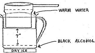
Tie the felt with a string around the top of the coffee pot and leave the felt loose enough so that the smaller pot can push it down till it is six or seven inches from the bottom. Sit the pot on the dry ice directly and connect the negative terminal of the battery to the felt where it is wet with methyl alcohol.
