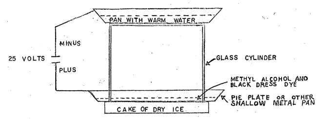
The hardest part to find is a glass cylinder which must be between 6 or 8 inches high, and more than 6 inches in diameter. The glass must be clear. The larger the diameter the better the setup works. We use 16 inch diameter cylinders. The wall thickness is not important.
