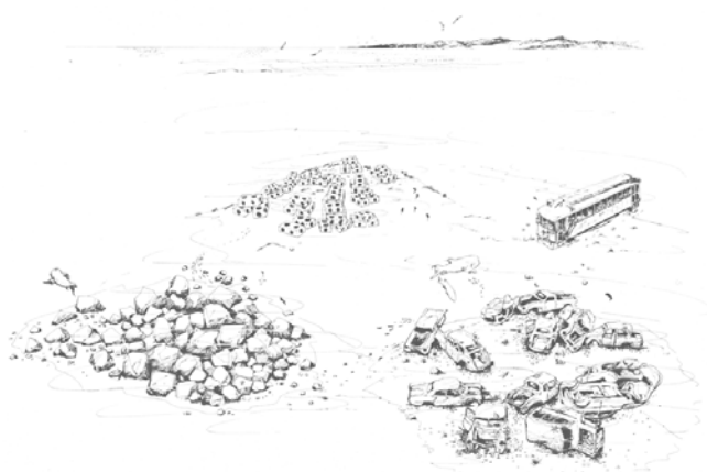
FIGURE 1 Artists concept of a multi-component study reef placed in Santa Monica Bay; 60-foot depth.
