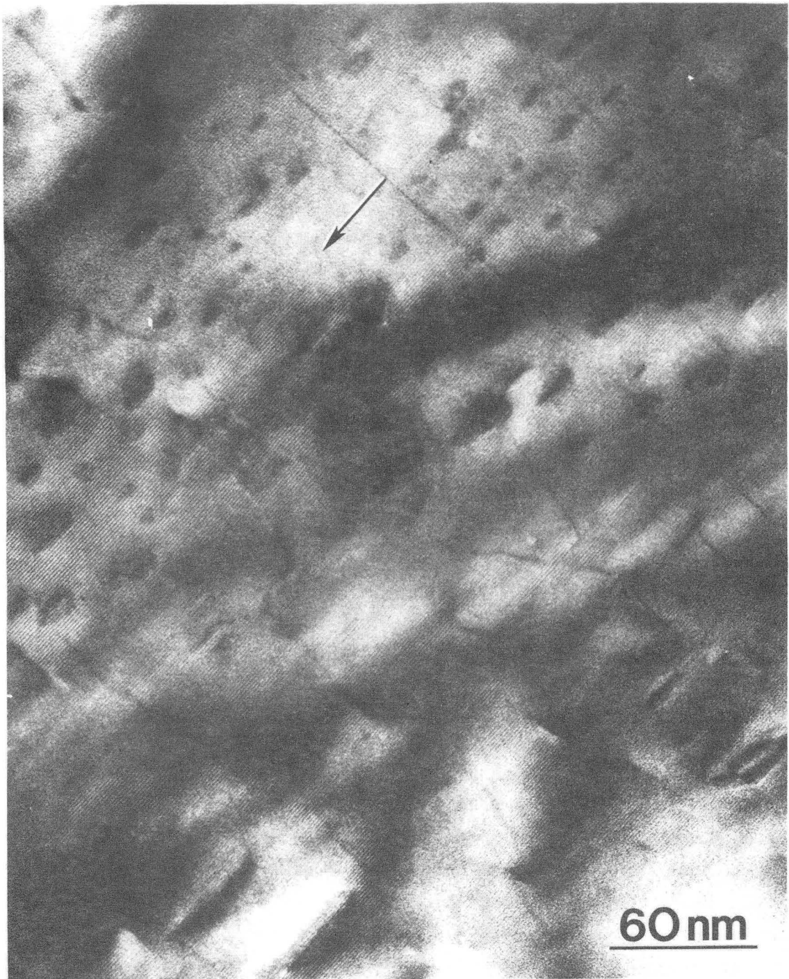
Fig. 10.10 HRTEM image of low chalcocite film in [010] zone-axis orientation. Note wandering (1/110) boundaries. Flat (1/110) boundaries are due to basal slip of sublattice dislocations. Arrow indicates [001] direction.
