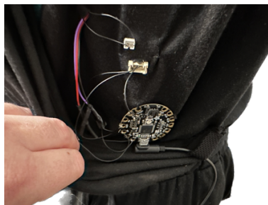
Figure 36: The microcontroller, Adafruit Flora, is embedded. The circuit is built using wire wrapping wire.
