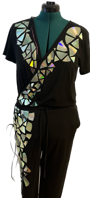
Figure 35: My wearable second skin. It features a reptilian-like scale structure made of CDs, galvanic skin response sensing, respiration sensing, and heart rate sensing. Front view.
