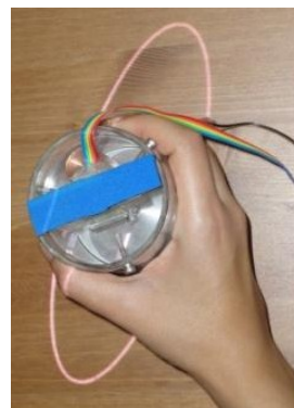
Figure 9. The device with a color marker on the top. The ellipse is augmented on the actual marker in real time by a projector.
