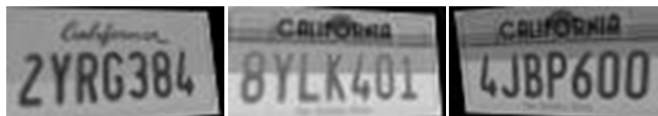
Figure 4.6: Examples of synthesized license plates. Notice how shadow lines and brightness level of the plate vary.
