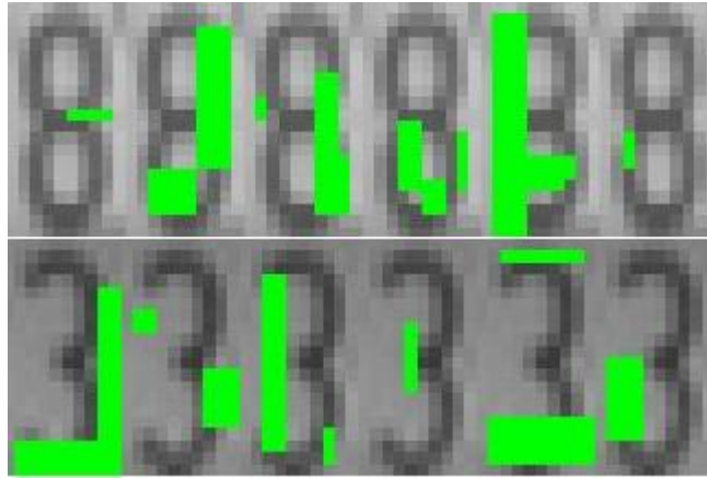
Figure 5.1: Shown above are the top features picked for a “3”, and a “8”. Notice that the fifth feature on the “8” is very similar to the third feature on the “3”
