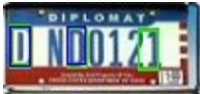
Figure 4.12: Example of a “D” Multiple Font classifier on a test image. Notice the fact that it detects “D” with different contrast in the same image and does not detect the “0”.
