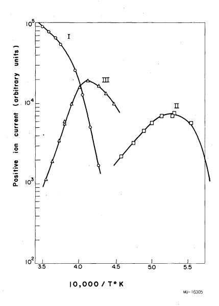
Fig. 19. Ionization of uranium on tungsten. Oxygen effect data taken as pressure of system slowly increased.
