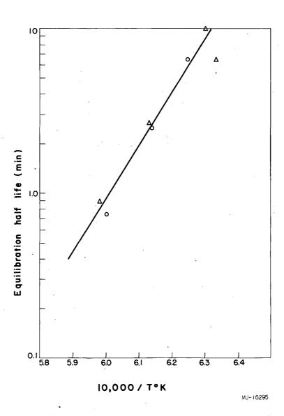
Fig. 9. Rate of equilibration of positive-ion current following increase in temperature.
