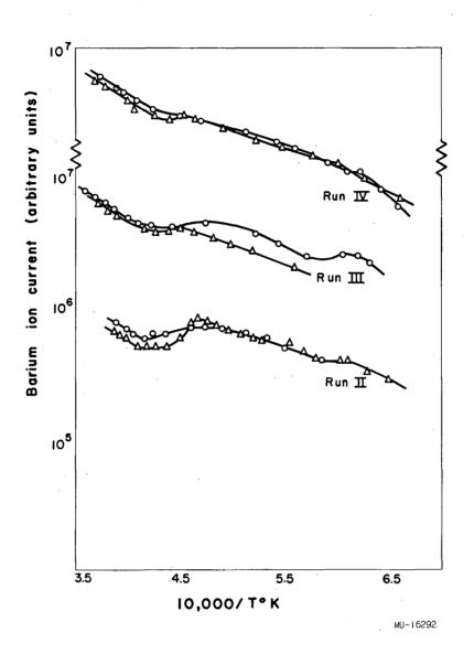
Fig. 6. Ionization of barium on tantalum.  $\Delta \quad \text{- Increasing temperature.} \\ 0 \quad \text{- Decreasing temperature.}$
