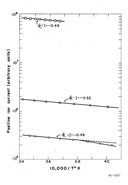
Fig. 21. Ionization of neodymium on tungsten; high-temperature region. Note: Vertical position of curves is arbitrary. Relative position is related to atomic-beam intensity.
