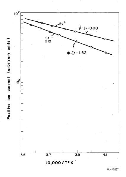
Fig. 11. Ionization of barium and strontium on tantalum; high-temperature region. Note: Vertical positioning of the two currents is arbitrary.
