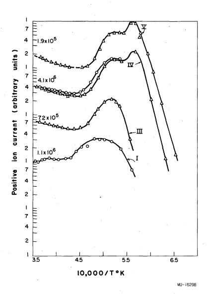
Fig. 12. The ionization of barium on tungsten.  $\Delta$  - increasing temperature O - decreasing temperature.
