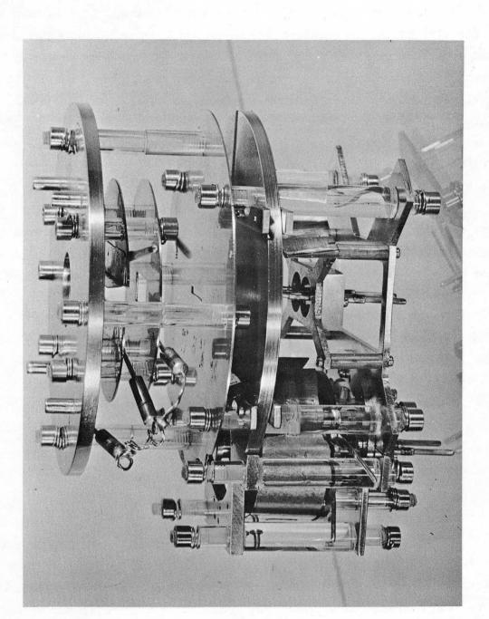
Fig. 4. Completely assembled ion source.
