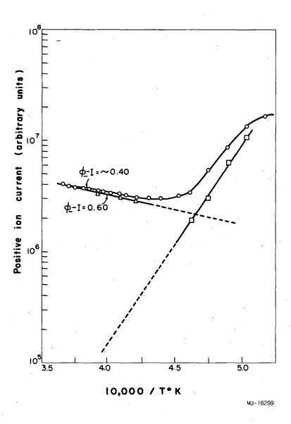
Fig. 13. Empirical resolution of Ba<sup>+</sup> current into high-temperature straight line and lower-temperature chemical effect.
