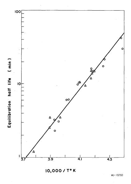
Fig. 7. Rate of equilibration of positive-ion current following increase in temperature.
