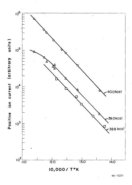
Fig. 5. Dependence of ion current on oven temperature,
