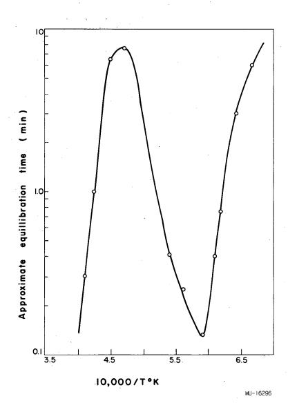
Fig. 10. Approximate equilibration rate; decreasing temperature; Ba<sup>+</sup> ion current on tantalum.
