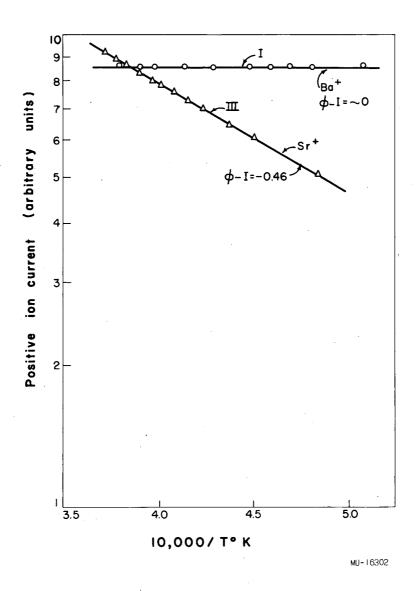
Fig. 16. Ionization of barium and strontium on rhenium; high-temperature region. Data corrected for drifts. Note: Vertical positioning of the two curves is arbitrary.
