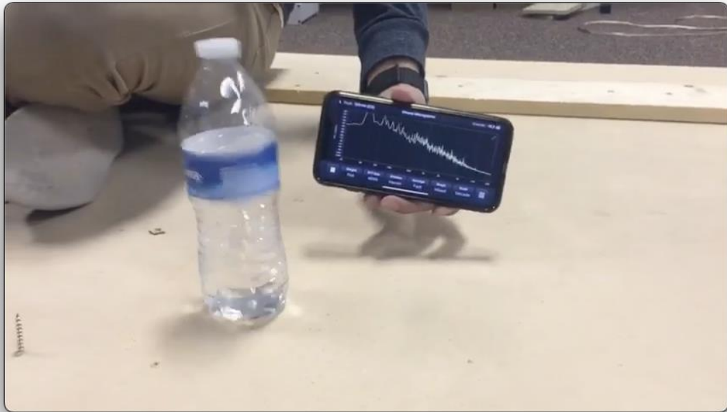
Figure 6: Water bottle responds to tactile stage, while FFT plot shows vibroacoustic response.
