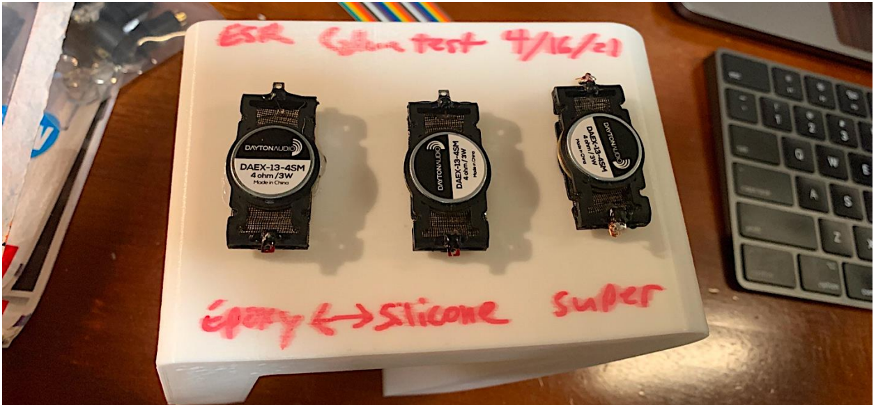
Figure 61: Glue test with exciters - epoxy and silicone labels were accidentally swapped - 4/16/2021
