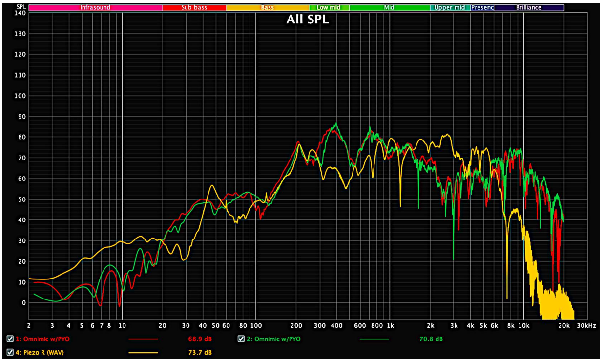
Figure 32: Room EQ Wizard Graph showing the combined frequency responses from the Piezo pickup, and the OmniMic V2 calibrated microphone
