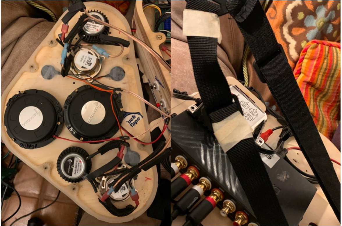
Figure 28: RX203 with three piezo pickups (left) the Dayton Audio DSP-408 joins the design (right)
