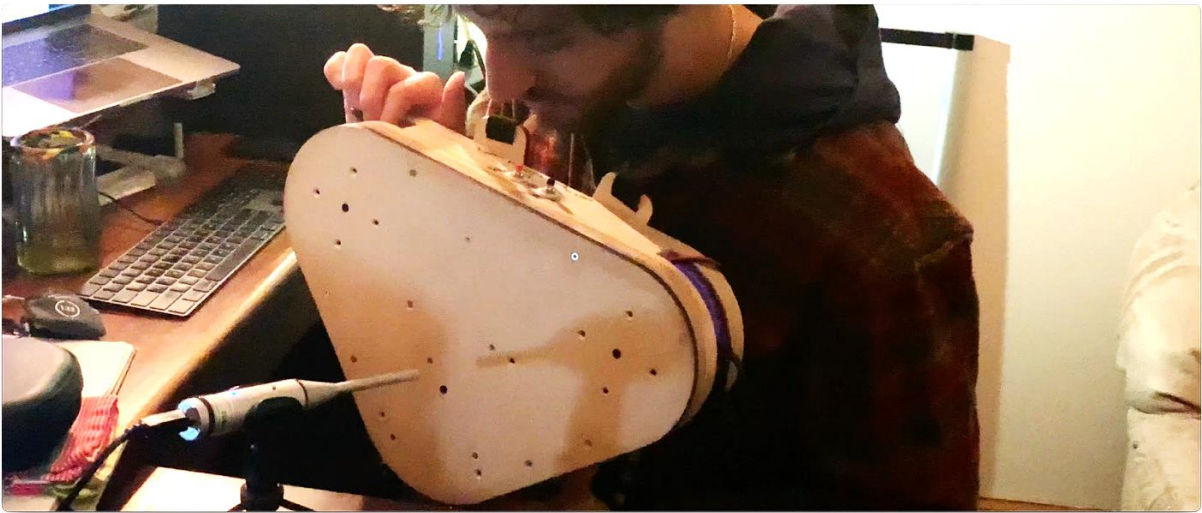
Figure 33: Screenshot of Ethan Castro testing the frequency response of the RX203 with a calibrated microphone. Taken November 24, 2020
