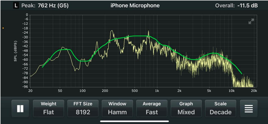
Figure 30: FFT plot capture of pink noise on RX202 device by iPhone XS Max microphone, with hand-drawn curve outlining frequency response of the device. Taken Nov 10, 2020
