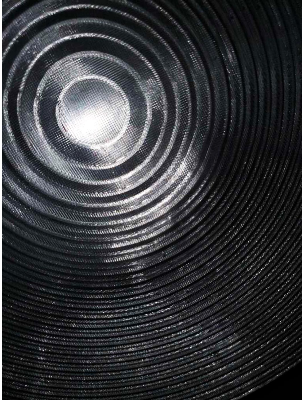
Figure 62: Close up of RX 304 deformations in the EP's external face, seen as dark spots and shadows
