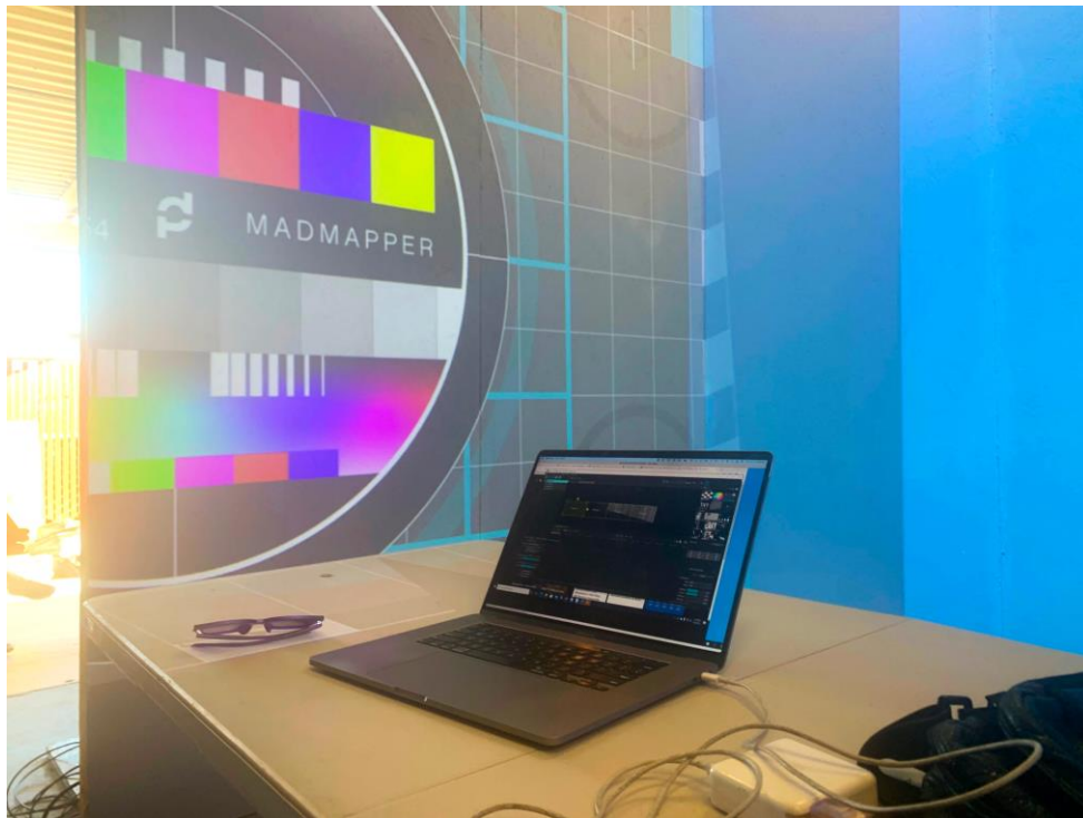
Figure 150: Software Madmapper being used to warp projector output to Aurora stage
