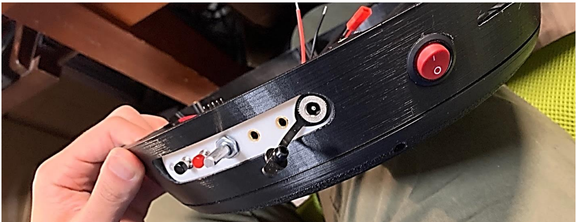
Figure 53: External view of RX300 I/O panel within the mid wall, missing knob on digital encoder
