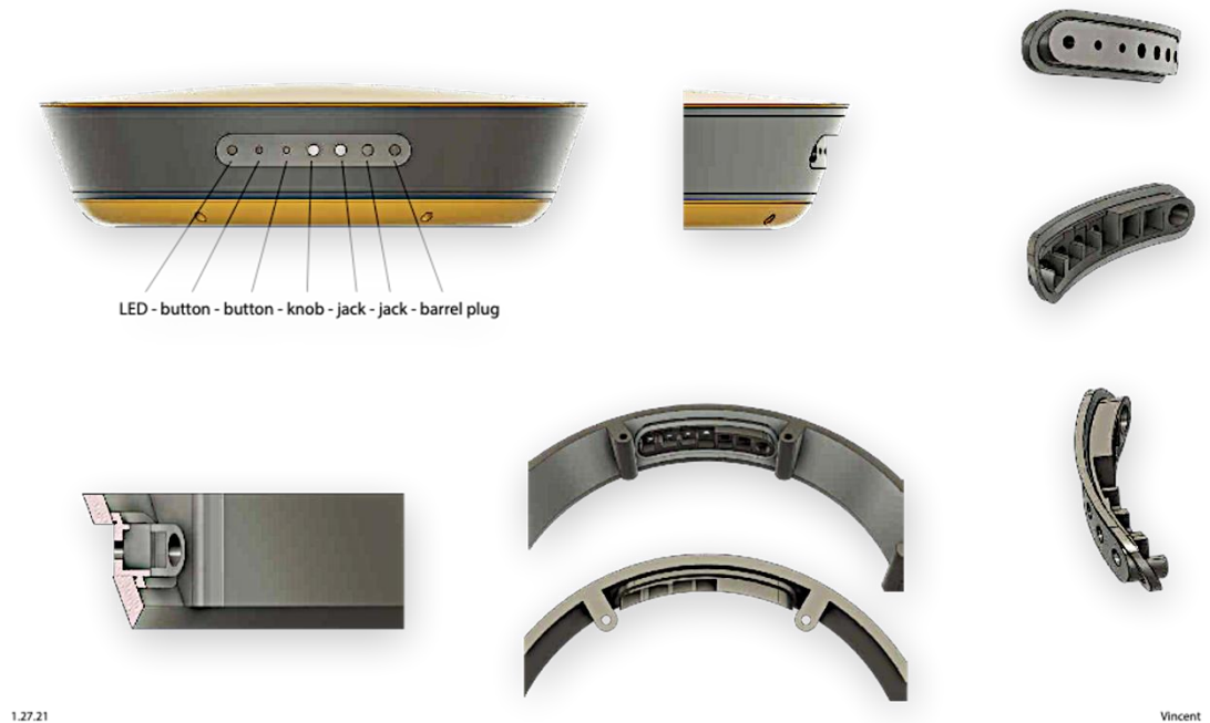
Figure 44: Renderings showing all the components that make up the RX 300 I/O schema
