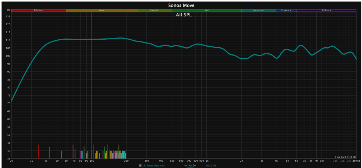
Figure 3: Frequency response of Sonos Move - contains one mid woofer and one tweeter
