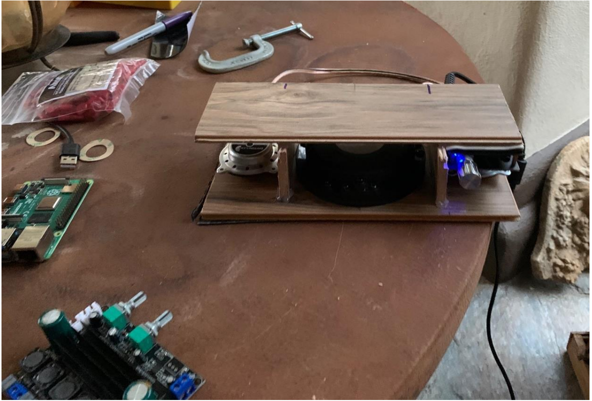
Figure 14: Photo showing assembled prototype miniature full frequency tactile audio module
