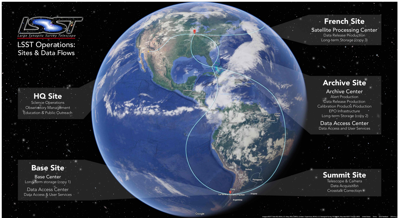
Figure 14. The LSST data flow from the mountain facilities in Chile to the data access center and processing center in the U.S., and the satellite processing center in France.
