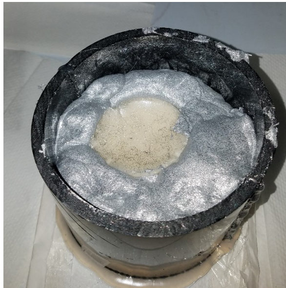
Figure 5.11.: The composite sample where a 60% Oil concentration sample is surrounded by a Al/TX-150 sample with 10 grams of Aluminum powder. Samples for measurement were taken from the middle of the Al/TX-150 sample, from the middle of the Oil Sample and finally from the interface between both samples.
