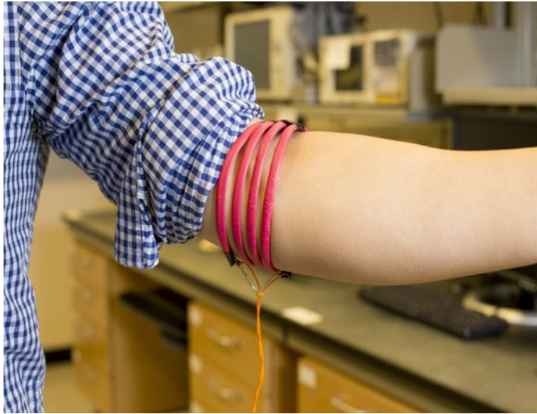
Figure 2.3: For each communicating node that will use the magnetic fields only approach as means for data carrier, a wrapped coil is need [203], where each node becomes really bulky in size, inconvenient and not efficient compared with wireless solutions in this case.
