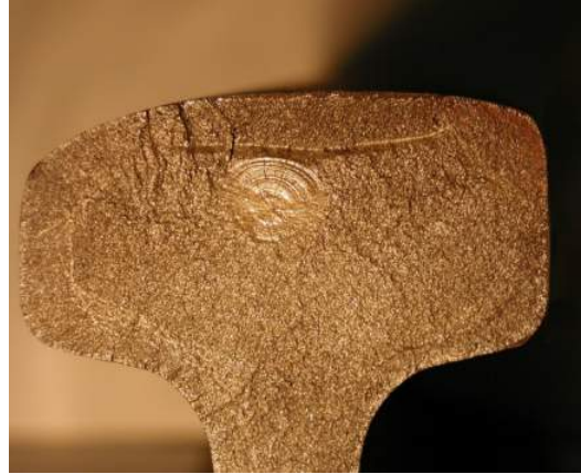
Figure 2.6: Example of a transverse fissure (Garcia & Zhang, 2006).
