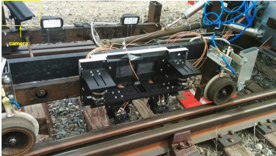
Figure 3.47: ENSCO Inc.'s camera mounted on the cart's frame.
