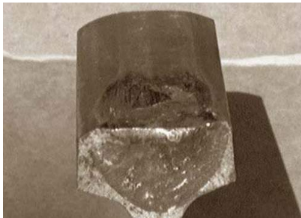
Figure 2.9: Example of a engine burn fracture (Garcia & Zhang, 2006).
