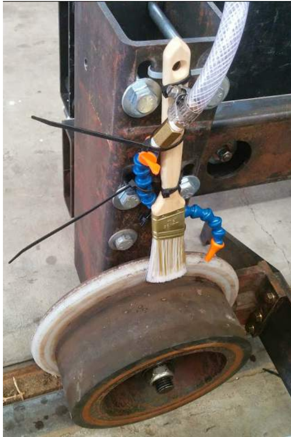
Figure 3.46: ENSCO Inc.'s water lubrication system. Here it is shown on one of the cart wheels.
