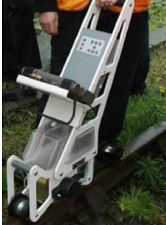
Figure 2.16: Portable "walking" ultrasonic wheel system (Clark, 2004).
