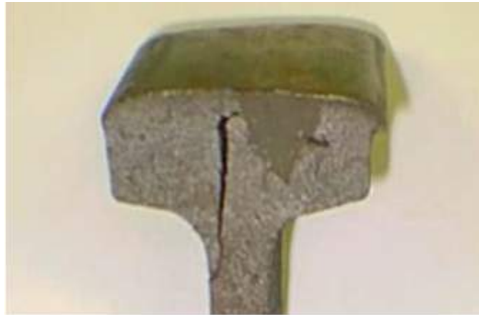
Figure 2.10: Vertical split head example (Garcia & Zhang, 2006).
