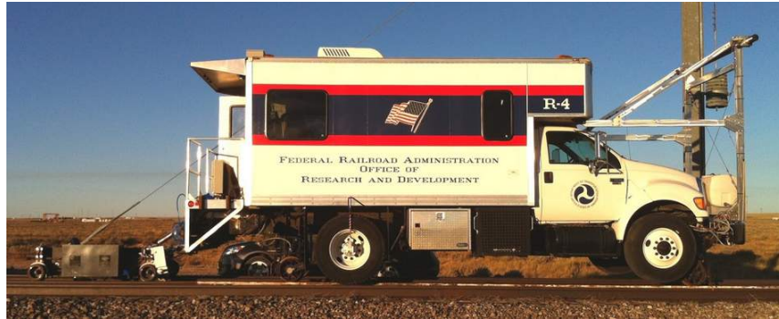
Figure 6.1: Rail defect detection system (pulled by a Hy-Railer).
