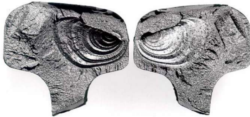
Figure 2.7: Example of a detail fracture (Garcia & Zhang, 2006).
