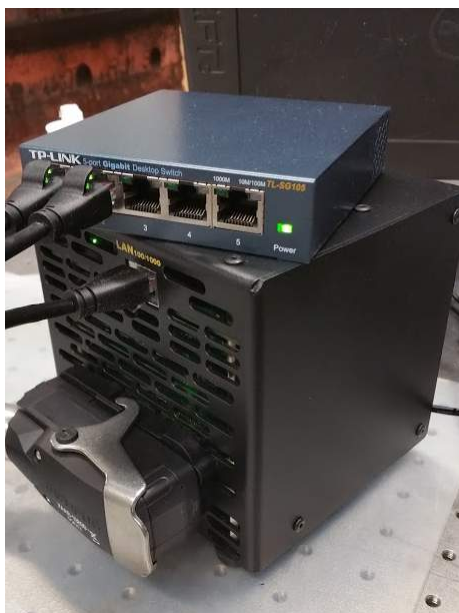
Figure 5.5: AOS analog-to-digital device and a gigabit Ethernet switch used to transfer data.
