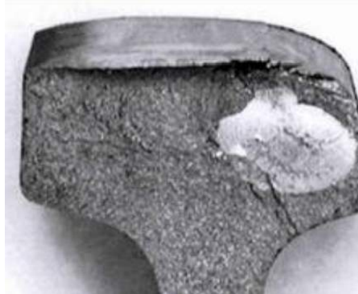
Figure 2.8: Example of a compound fissure (Garcia & Zhang, 2006).
