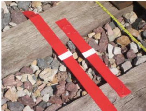
Figure 3.48: Reflector attached to the wooden ties.
