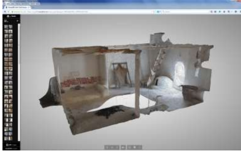
FIGURE 6 Image-based 3D model of Çatalhöyük Experimental House generated in Autodesk Recap 360
