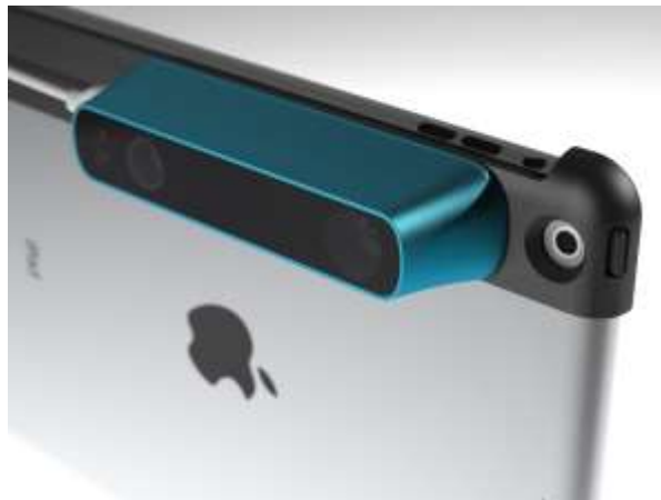
FIGURE 1 Structure Sensor uses iPad for real-time data processing - Courtesy of Occipital
