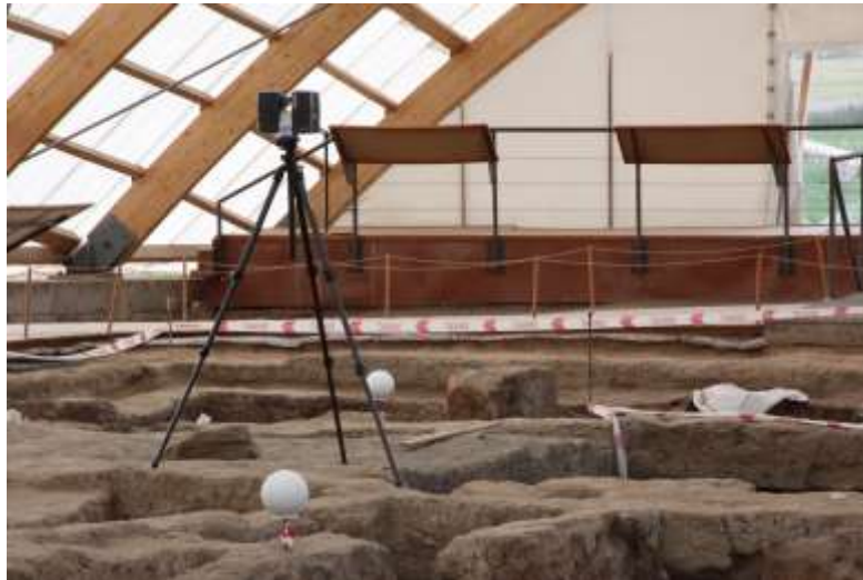
FIGURE 8 FARO Focus S120 scanning Neolithic buildings in the North Area at Çatalhöyük, East Mound
